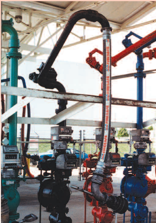
FIRESAFE HOSE STILL INTACT AFTER 30 MINUTES OF FIRE.
