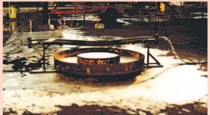
FIRESAFE HOSE STILL INTACT AFTER 30 MINUTES OF FIRE.
