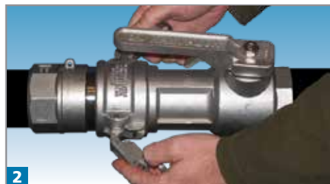
2 Cam Arms Lock Coupler and Adaptor Together
